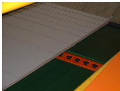
Separation conveyor with vacuum bar
